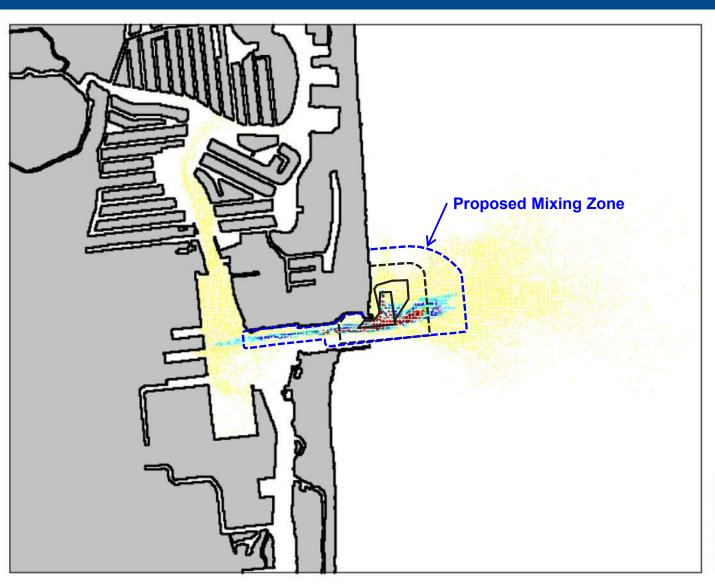
Thickness of sediment deposition (mm) -Dredging at Sand Trap
