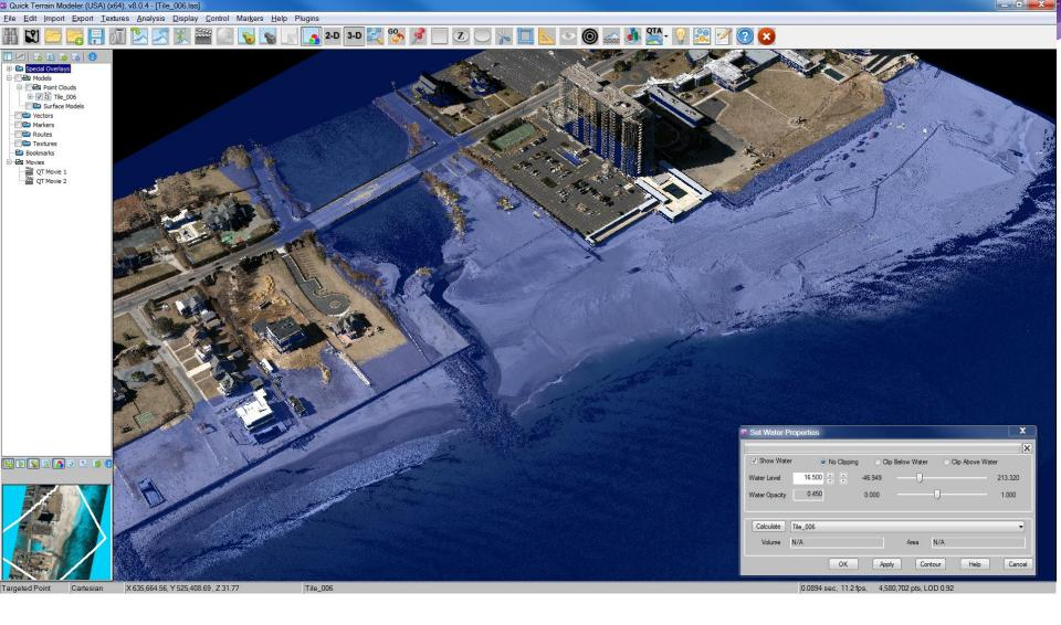
Surge Model Using a Colorized Point Cloud
