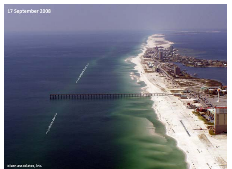
Figure 3 Aerial view of Pensacola Beach following Hurricanes Gustav and Ike. Note the broad accumulation of sand in the nearshore zone and the uniform position of the offshore bar, which was pushed 150 to 200 ft farther offshore during the storms (nearly to the end of the Pensacola Beach Fishing Pier (ES R-120)).
