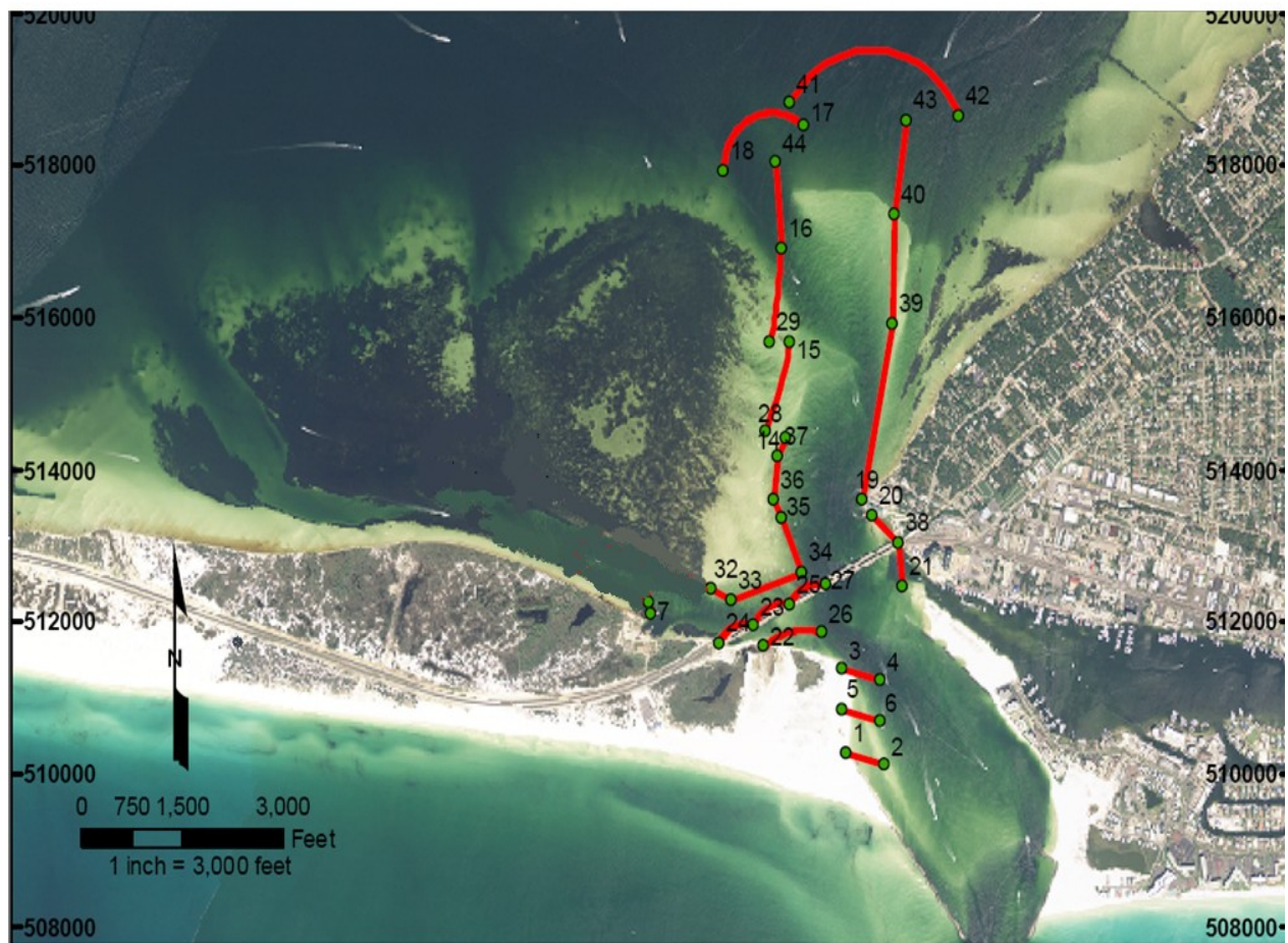
Figure 5. Boom plan north of Destin Bridge. Boom is placed and aligned so that relative currents are less than 0.7 knots.
