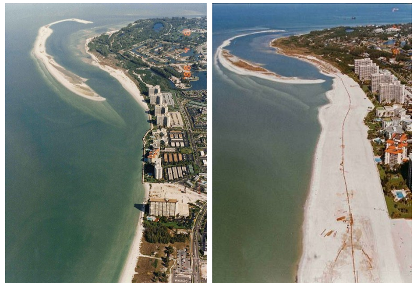
Marco Island Nourishment, Before and After Photos Courtesy of Coastal Engineering Consultants, Inc.
