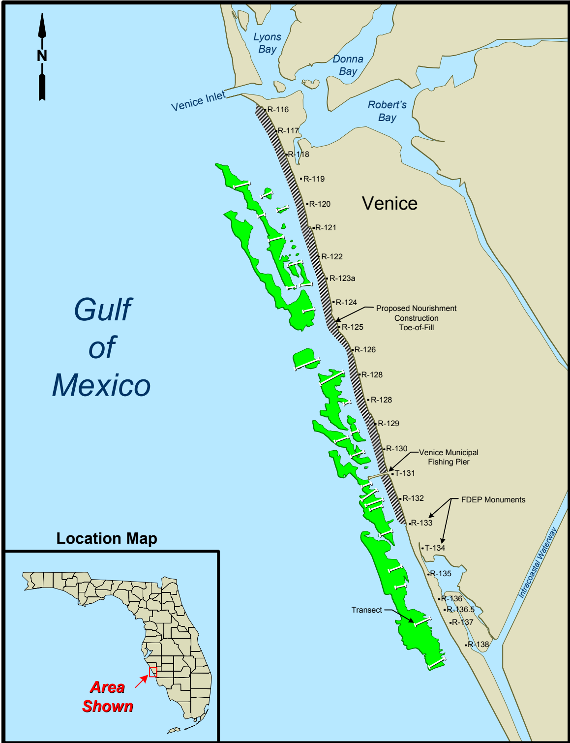
Figure 3. Placement of transects on nearshore reefs for monitoring the City of Venice beach nourishment project.
