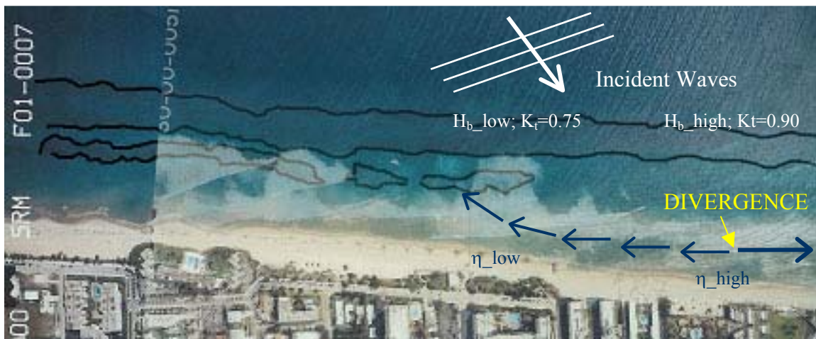
Figure 6: Description of circulation system at Hillsboro and Deerfield Beach. The variation in breaking wave height induces an alongshore variation in wave set-up at the shoreline. This variation creates a sea-surface slope down toward Deerfield Beach. The sea surface slope induces a pressure gradient toward Deerfield Beach, and water and entrained sediments will tend to move toward Deerfield Beach. The current induced by the variation in alongshore sea-surface elevation must be added to the current induced by waves arriving to the shoreline at an angle.
