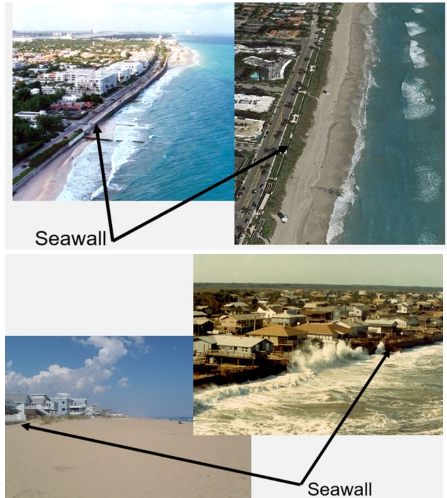
Figure 4. Multiple renourishments developed robust dunes and sandbars in areas that were historically fronted by seawalls.
