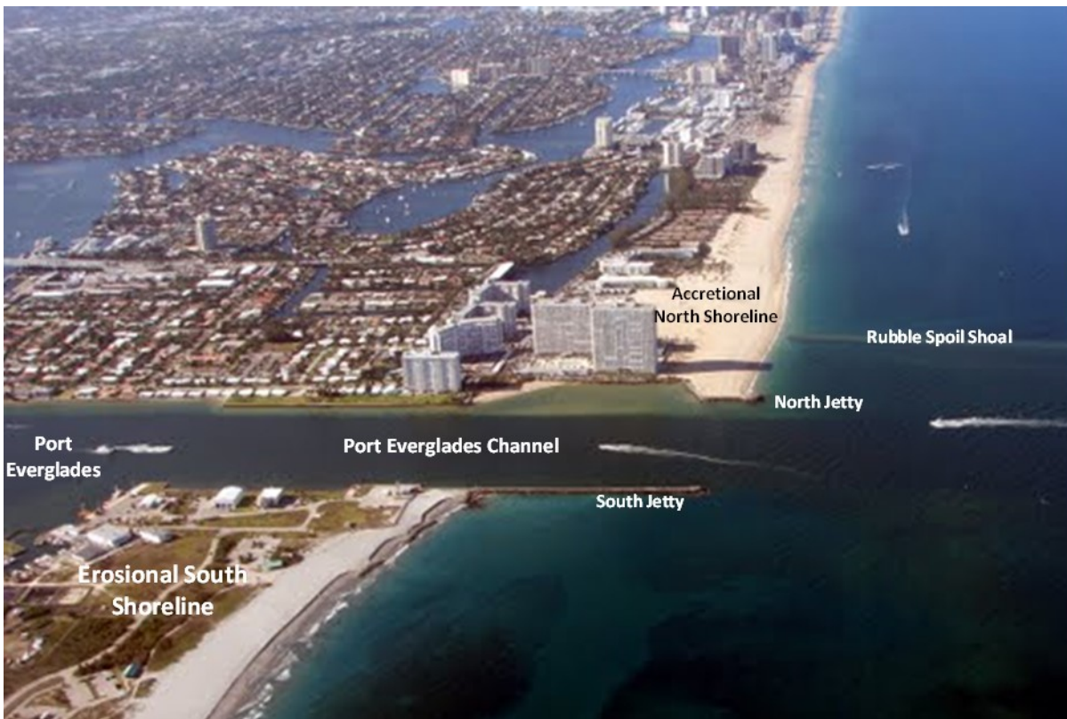
Existing configuration of inlet and adjacent shorelines, looking northward. This vantage point demonstrates the significant shoreline offset across the inlet.
