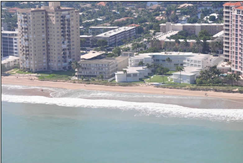
Figure 1: Loss of berm width and height, scarping into dune line following the passing of Hurricane Sandy. Photo taken at Bel Aire Drive, northern Lauderdale-by-the-Sea on 10/29/12.
