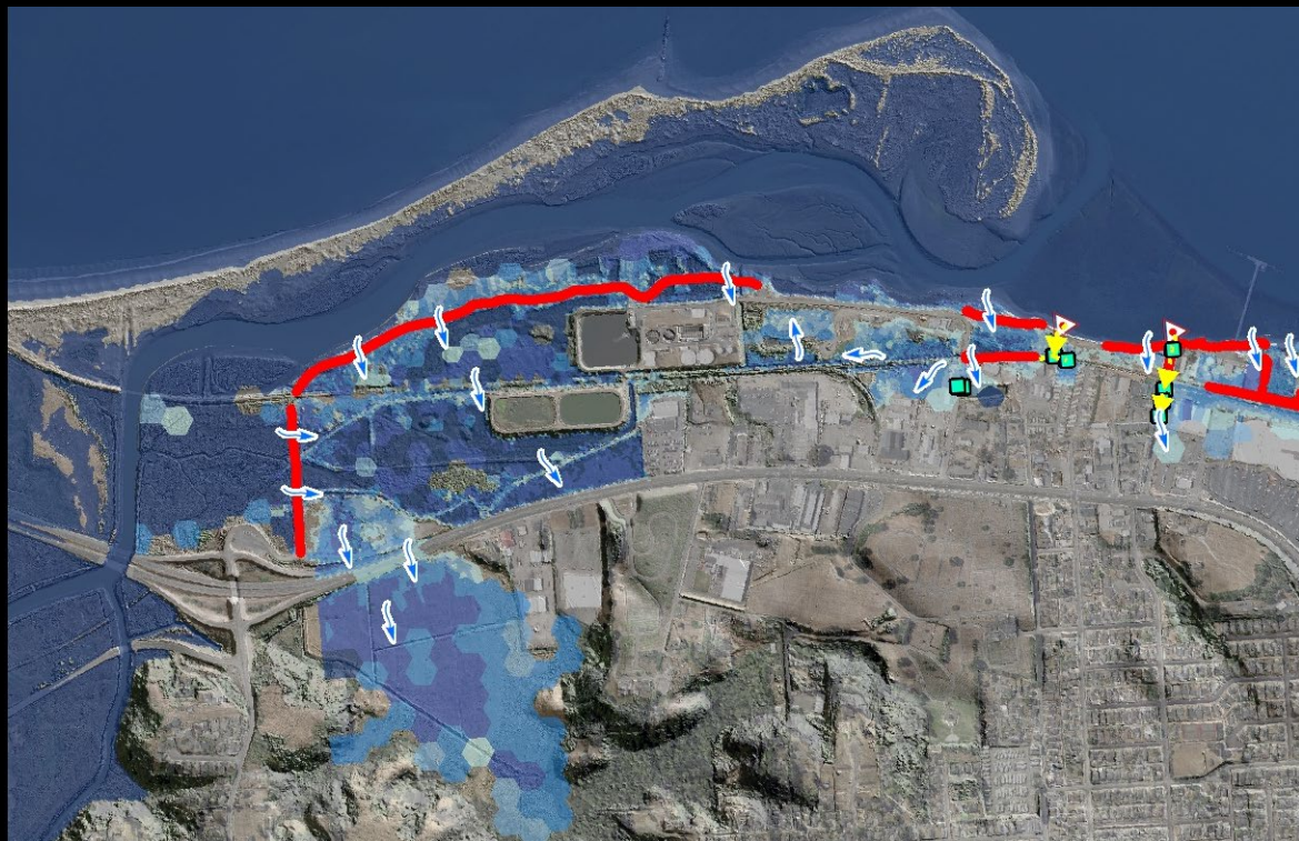
Existing Pathways of Inundation and Depth of Flooding
