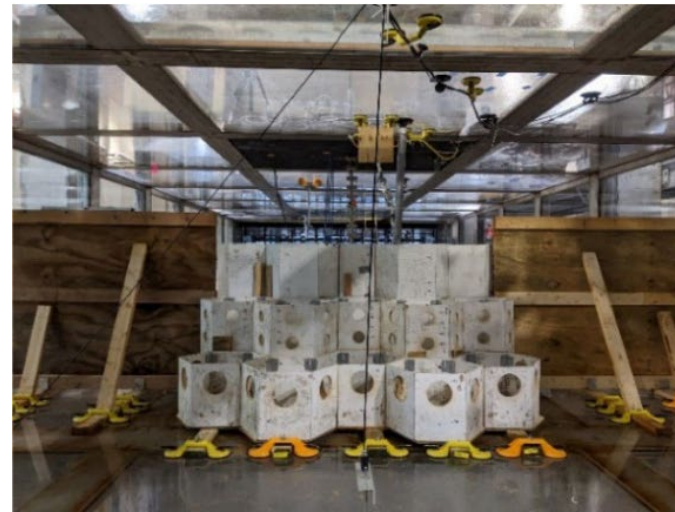
FIGURE 11 Semi-perforated SEAHIVE system model configuration in SUSTAIN.
