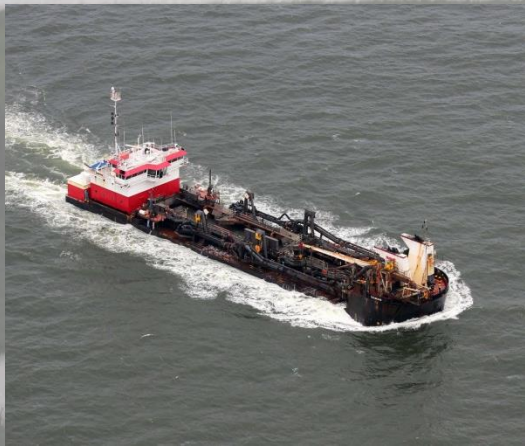
Hopper Dredge Excavation and Transport to Fill Area
